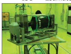
Device to rotate RANDO phantom Simulation of isotropic irradiation
